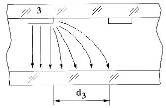
*Figure 2. The construction of deflector on wedge-shaped deformation with system 3 electrodes.*
