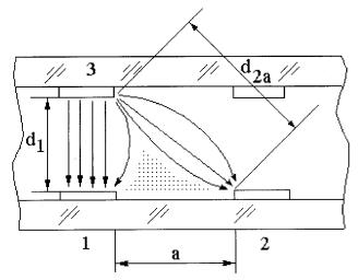
Figure 1. The construction of deflector on wedge-shaped deformation with system 4 electrodes.
