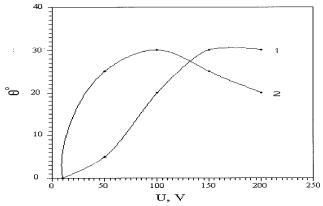
*Figure 4. The angle deflection and applied voltage dependence for the deflectors on diffraction structures*
