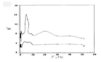
Figure 3. The frequency dependence of angle deflection for a deflector on diffraction structure.
